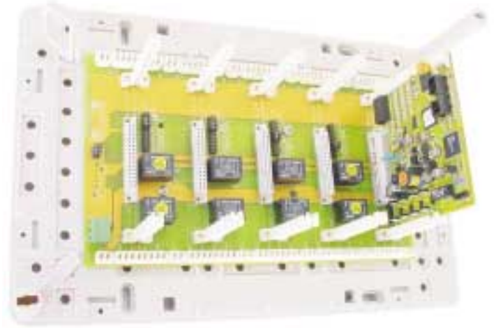
Remote Motherboard Enclosure
